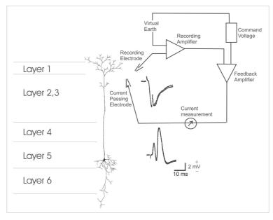
Figure 6. Schematic showing principles involved in voltage clamping LFPs.
